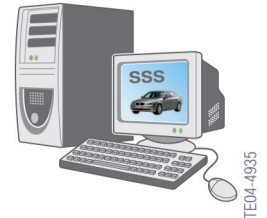
Control units can now only be programmed with the Software Service Station.
